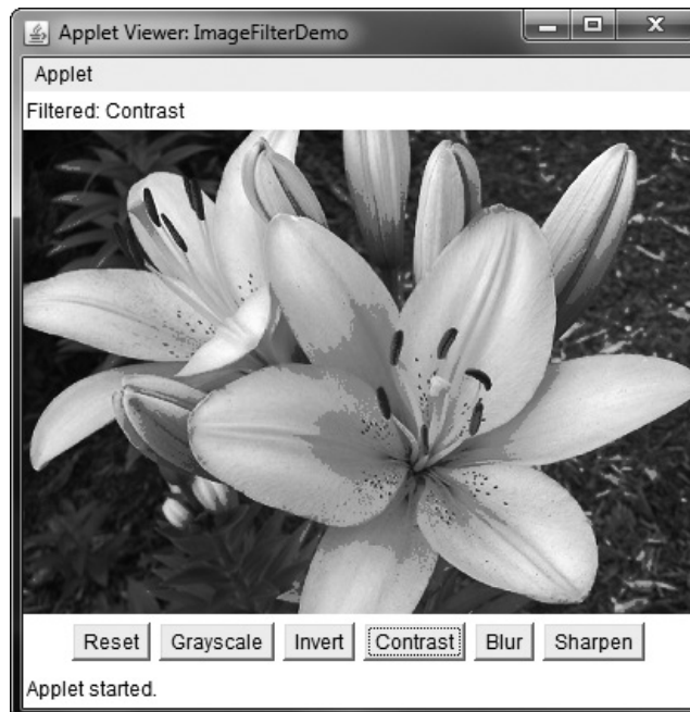
Figure 27-8 Using the Contrast filter with ImageFilterDemo
