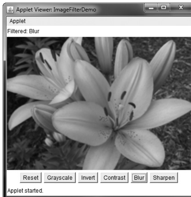
Figure 27-9 Using the Blur filter with ImageFilterDemo
